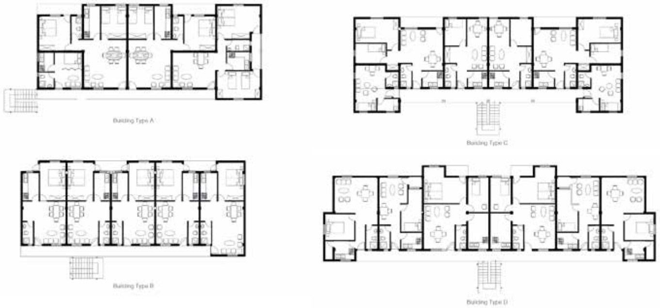
Figure 3: Building types and typical floor plan for the Bole-Gerji pilot project. Source: Construction Ahead, 2005
