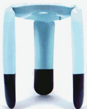
The Stool , the idea was to produce stable and convenient furniture out of thin metal sheets using the potential of CNC machines and hydro formed metal surfaces. The hydro-formed process applies liquids with high pressure to the water-tight welded inner space. This pressure and the thickness of the metal sheets define the 3D appearance and stability of the chair. Design: Oskar Zieta www.zieta.pl
