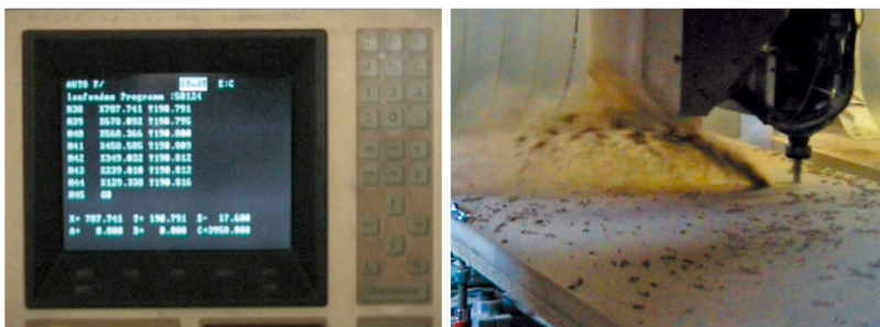
Figure 5: The generated code for the 5-axis router is directly fed into the machine without manual revision. The three CNC-fabrication steps are: Drilling: crating dowel holes for the connections Roughing: pre-cutting the form of the rafters Finishing: smoothing the surfaces
