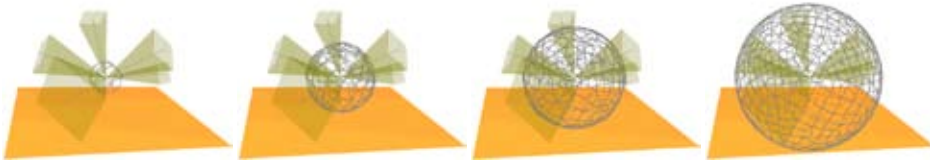
The mesh of the Swissbau sphere is dynamically "growing" in an interactive simulation. The edges are aligning to the windows (green) and the floor (orange).
