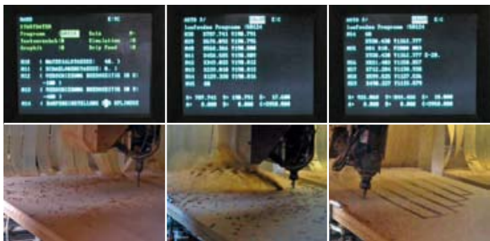
The code for the 5-axis mill is directly fed into the machine without manual revision. The three CNC-fabrication steps are: Drilling: crating dowel holes for the connections Roughing: pre-cutting the form of the rafters Finishing: smoothing the surfaces
