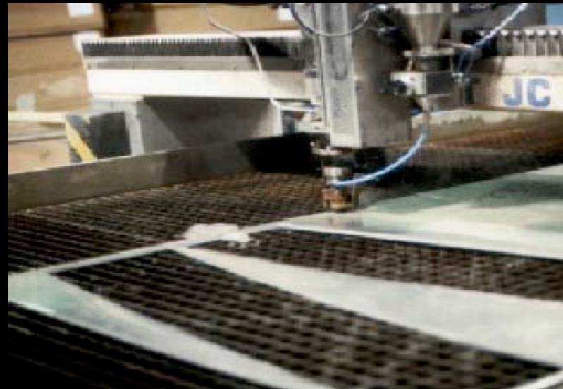
Aluminum space frame for ABB Architects' BMW Pavilion is cut directly from digital data using CNC water-jet technology.
