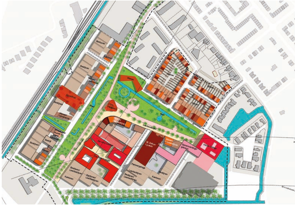
Master plan of Leer Park showing the mix of education and sports facilities, offices, retail, housing and multipurpose and open spaces.
