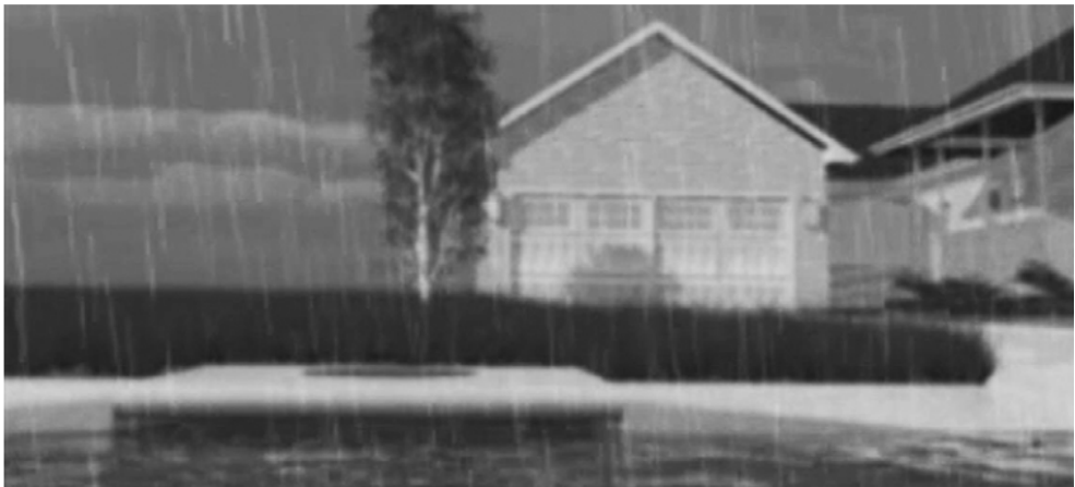
Fig. 5: Low-res video frame from a Vue simulated rain event where depth of gutter flow and water color (pollution) was approximated from GIS-based hydrology.
