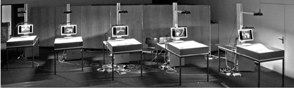
Fig. 3: Workshop laboratory showing 5 modelling stations consisting of the sandbox, a display, the 3D scanner and a computer.
