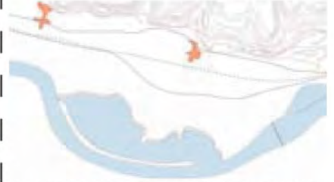
low-level polder excavated deep and maintained mostly empty
