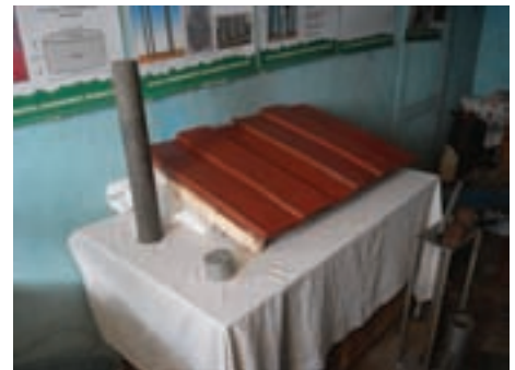
Recycled roof tiles and fencing poles
