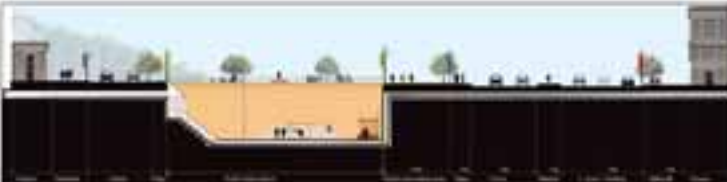
Illustration 7.7: Section through main East-West connector: Street below-grade
