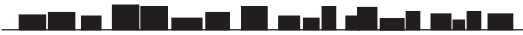
Dense irregular network Very narrow enclosed streets Buildings detached with very small gaps 1-2 floors
