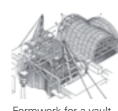
Formwork for a vault
