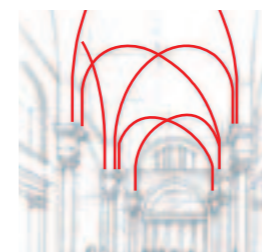
The Groin Vault - An intersecting Barrel vault
