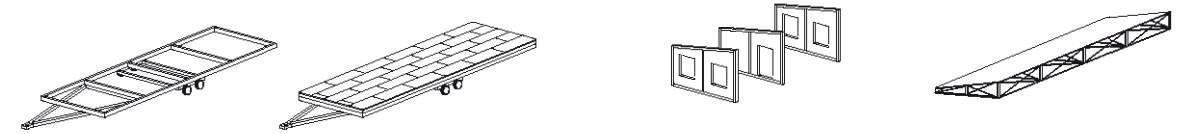
First, workers cover a reproduced steel frame with an insulated floor
